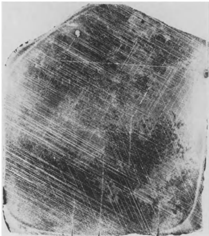
Fig. XIV-11. Polished and etched section of Edmonton (Canada) hexahedrite, like all large-crystal hexahedrites, a member of group IIA. The fine lines are called Neumann lines and are mechanical twins produced by low-pressure shock. The irregularly round inclusions are troilite. Small, white needles are schreibersite crystals in the rhabdite form. The density of rhabdites is quite variable. The specimen is about 9 cm wide. (Smithsonian Institution photo)
