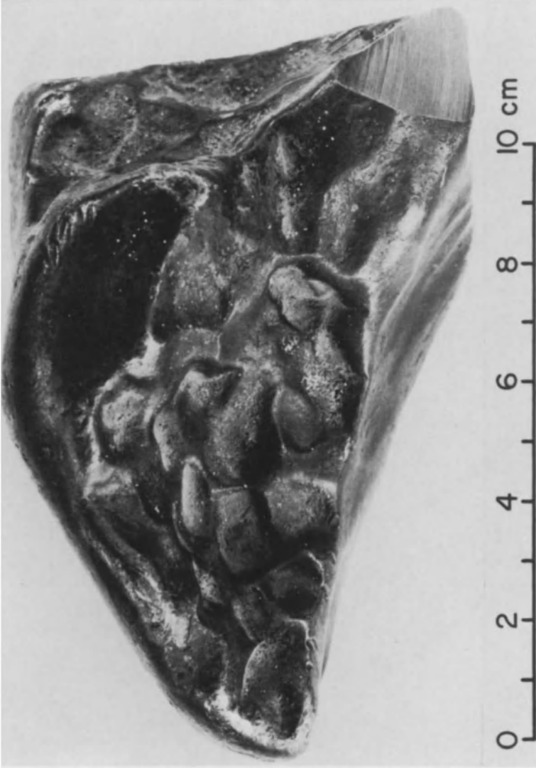
Fig. XIV-1. Exterior of the IV A iron, Bushman Land. The shallow depressions and polished appearance of the surface are typical of fresh iron meteorite falls. A small sample removed from the lower left corner shows a well-preserved heat-alteration zone and confirms that this meteorite find is a recent fall. (Smithsonian Institution photo)
