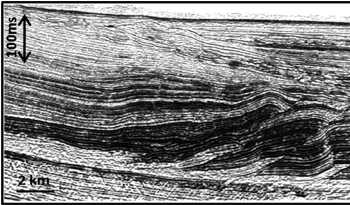
Fig. 4.9 A seismic segment showing an example of imbricate structures formed in extension regime. Gravity sliding of huge mass of mobile shale due to slope failure causes a buttressing force (compression) within the shale that results in forming imbricate structures. Also called “gravity tectonics” it must be distinguished from imbricates formed in compressional tectonics regimes (Image: courtesy ONGC, India)
