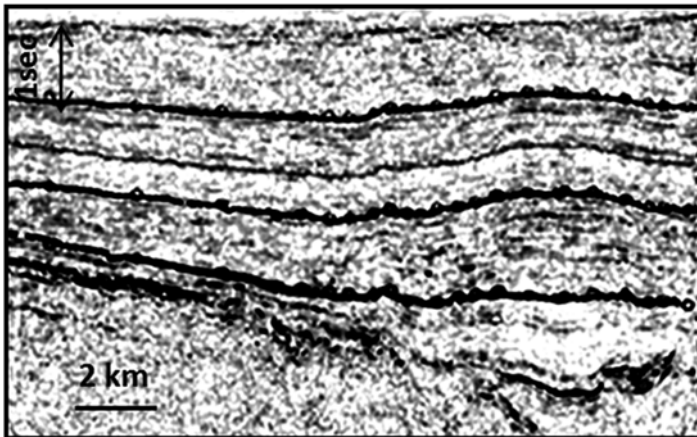
Fig. 4.18 A seismic segment showing an 'Inversion' structure associated with wrench typified by a synform vertically overlain by antiform (Image: courtesy ONGC, India)
