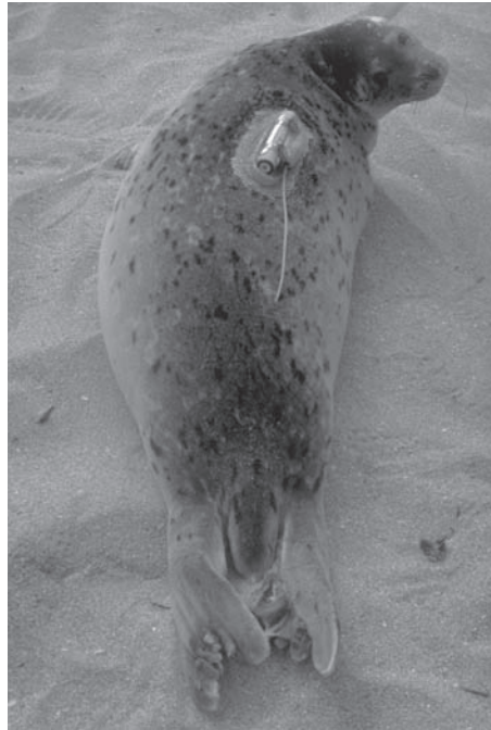
Figure 3.12. Harbor seal with TDR glued to skin and rear flipper tags (courtesy B. Stewart, Hubbs–Sea World Research Institute).
