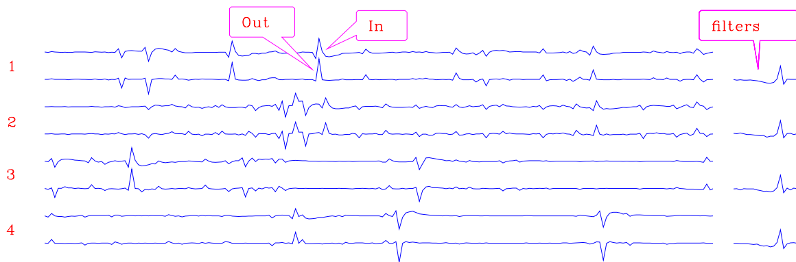
Figure 7.14: Four independent trials of deconvolution of sparse noise into an all-pass filter. Alternate lines are input and output. tsa-dallpass [NR]
