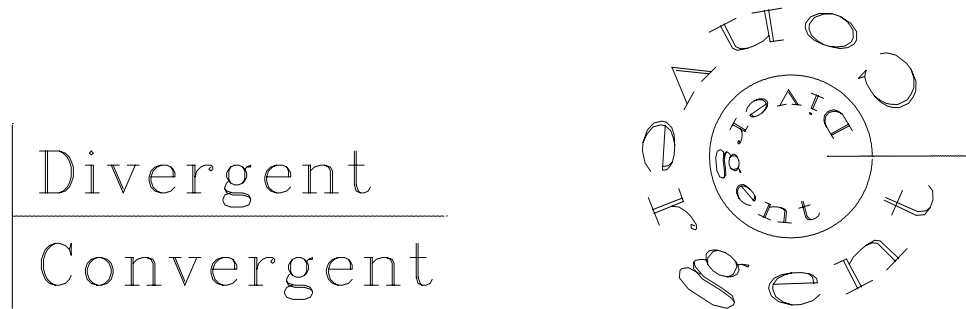
Figure 3.12: Left is the complex \omega -plane with axes (x, y) = (\Re\omega_0, \Im\omega_0) . Right is the Z -plane with axes (x, y) = (\Re Z_0, \Im Z_0) . The words “Convergent” and “Divergent” are transformed by Z = e^{i\omega} . zp-Z [ER]
