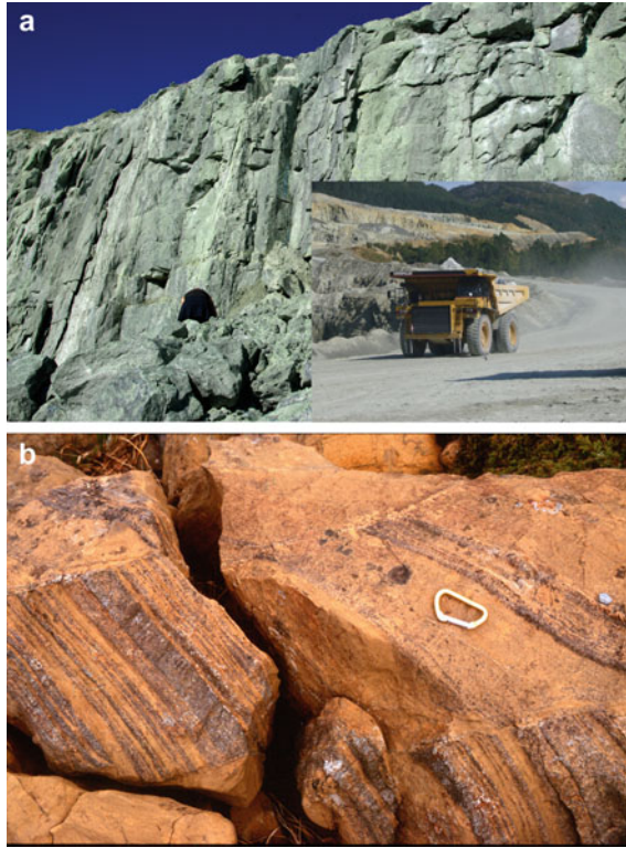
Fig. 5.1 a World largest olivine (dunite) mine, Almklovdalen, Norway. Alpine type peridotite in Caledonian continental basement. The 8 m high benches in the quarry consist of coarse-grained pure olivine (forsterite) rock. b Layered peridotites in gabbro magma chamber. Leka Island, Norwegian Caledonides. Note typical yellow–brown weathering crust on peridotite matrix
