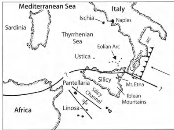
Fig. 3.64. The Eolian Island arc in the Tyrrhenian Sea. Volcanic activity in this tectonically complex area is caused by interactions between the African and the Eurasian Plates. The Eolian Island arc has formed as a result of subduction of the African Plate, whereas the volcanic activity on Sicily (Mt. Etna, Iblean Mountains) and in the Sicily Channel (Pantellaria, Linosa) is the result of crustal extension (Source: adapted from Barberi et al. 1973)
