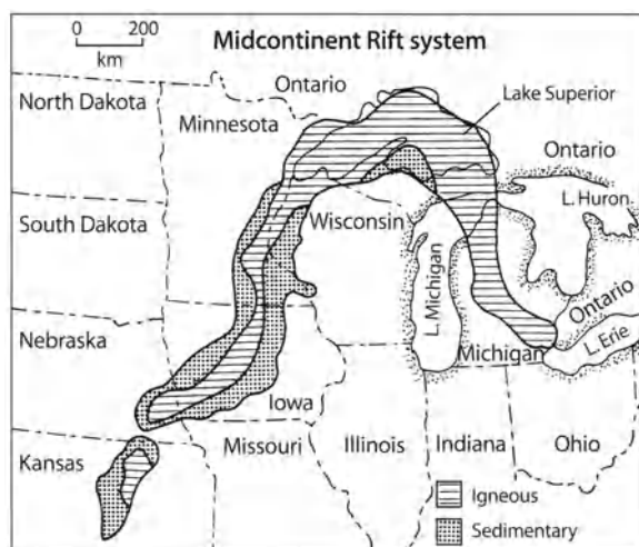
Fig. 7.1. Midcontinental Rift system of North America containing tholeiite lava flows with minor rhyolite, interbedded conglomerates, sandstones, and shales as well as differentiated gabbroic and alkalic intrusives. These rocks were deposited within a failed rift system at about 1100 Ma and are exposed in the Lake Superior area (Source: adapted from Van Schmus et al. 1987 and Nicholson et al. 1992)
