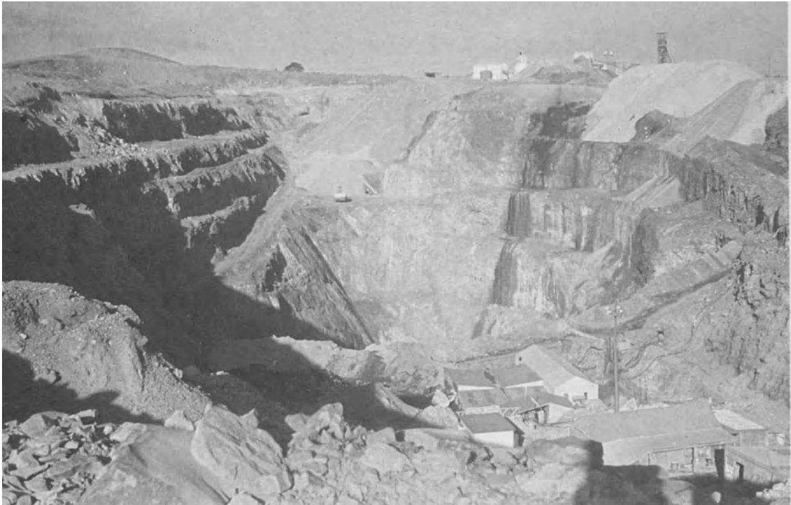
Fig. 6.22 The open pit at Tynagh from which oxidized ore was exploited. Note that the Tynagh fault plane defines one side of the pit.
