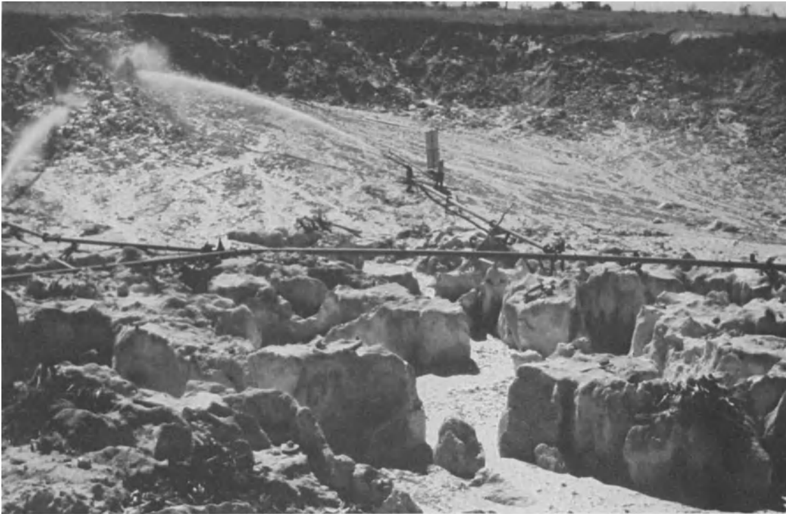
Fig. 5.8 Gravel-pump mining alluvial tin in the Kinta Valley, Malaysia. Note the karstic topography of the limestone below the alluvium. High tin values commonly occur near the limestone/alluvium interface, tin here can be recovered most effectively by reducing the alluvium to a slurry. The slurry is then pumped to a gravity separation plant.
