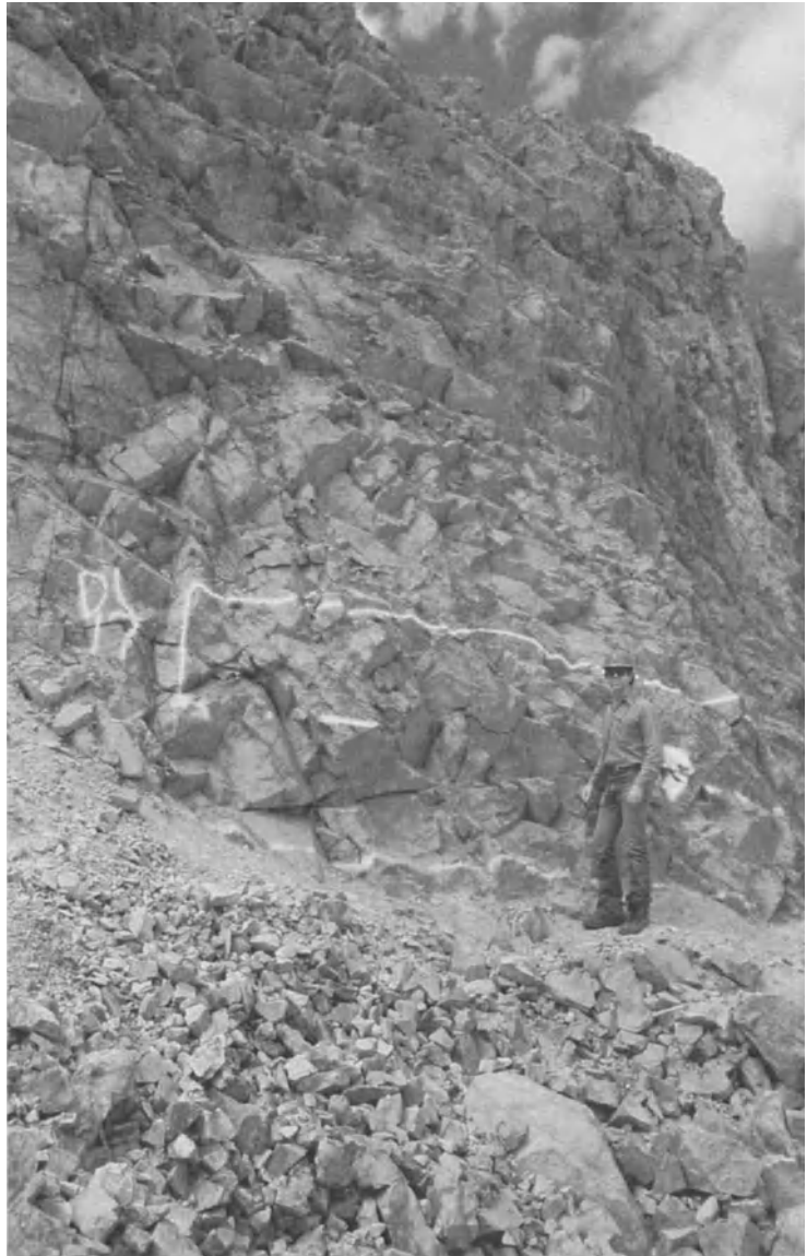
Fig. 3.15 Fracture analysis is important in porphyry deposits, not only during exploration but also in stability analysis of operating open pits such as here at Morenci Mine, Arizona.
