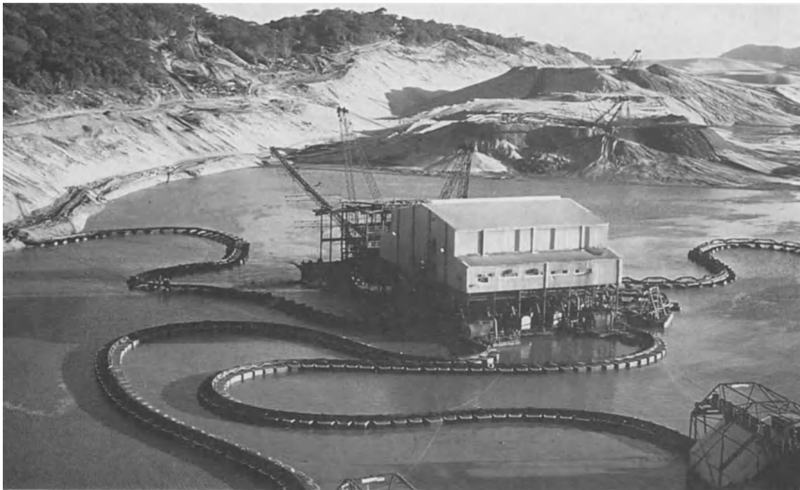
Fig. 5.19 A concentrator separating valuable heavy minerals from an unconsolidated aeolian sand. Richard's Bay, Natal, South Africa.
