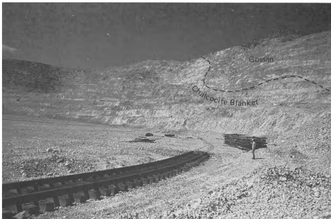
Fig. 3.13 Morenci Mine, Arizona. At the end of the 19th century a small underground operation here was producing copper at grades approaching 20%. Part of the supergene-enriched blanket is still visible overlain by the extensive gossan.
