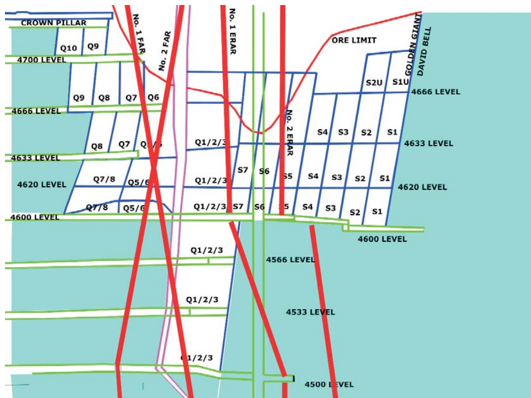
FIG 9 - Long-section of the shaft pillar ore zone and surrounding infrastructure (looking north) (MacMullan, Bawden and Mercer, 2004).
