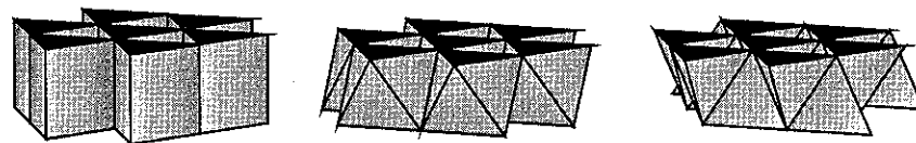
Fig. 6.37. From left to right: parts of layers of trigonal prisms, octahedra and tetrahedra.
