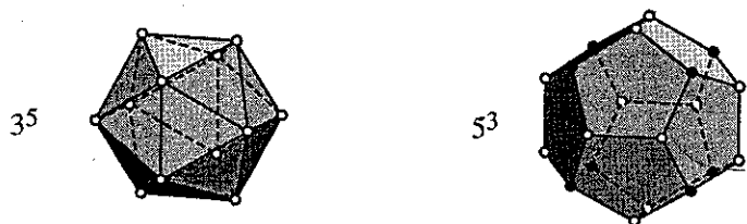
Fig. 5.2. An icosahedron, 3^5 (left), and a dodecahedron, 5^3 (right). Broken lines are edges obscured by the front faces.
