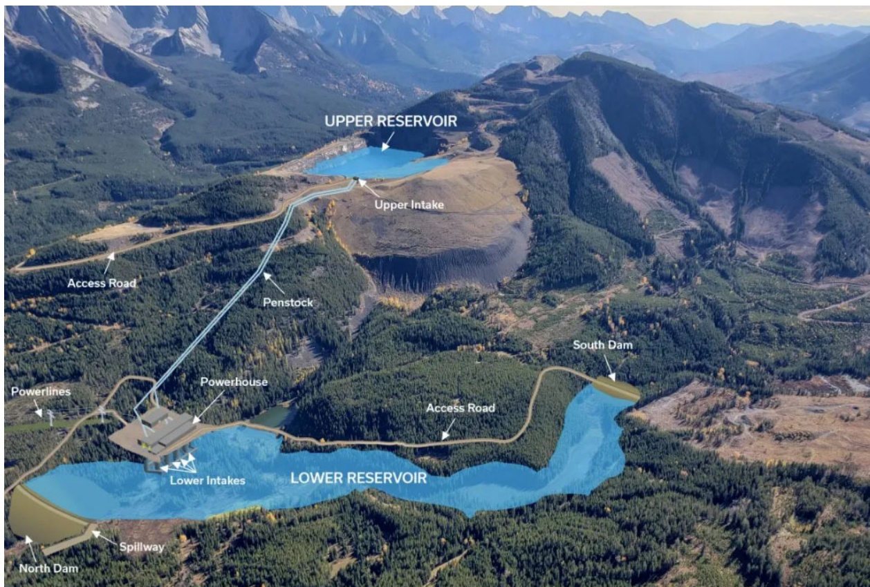
FIG 2 – Overlay rendering of the PHES configuration at Tent Mountain (courtesy of Montem).
