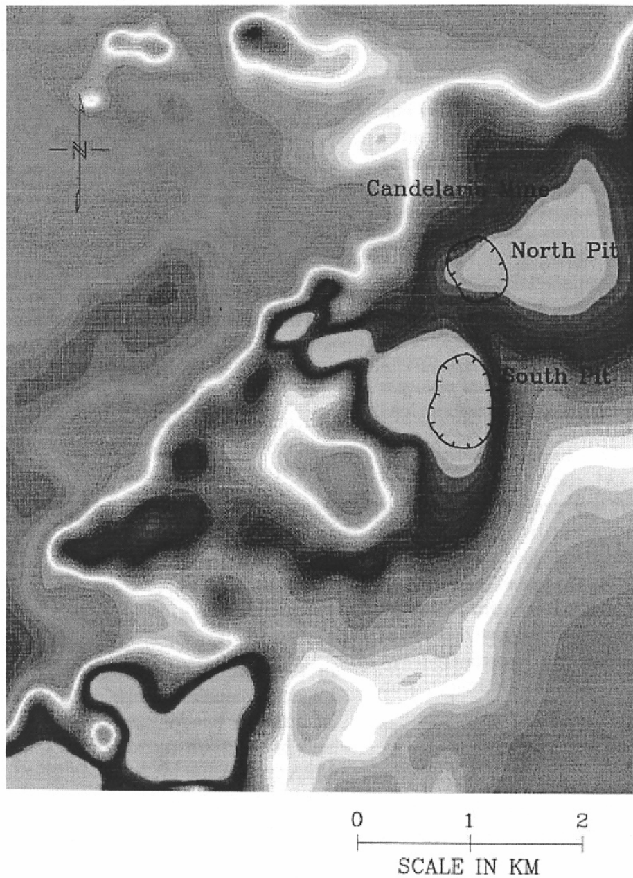
Figure 16. Airborne magnetics (reduced to pole) for the Candelaria Cu-Au deposit (from Smith, 2002).
