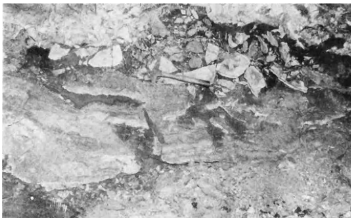
Fig. 5. Gray dolomite blocks (medium gray) with bottoms and sides fringed by pink dolomite (light gray) in a matrix of banded jasperoid (dark gray). Sphalerite (speckled gray) is concentrated in the jasperoid above the blocks. M bed, Lucky Jew mine.
