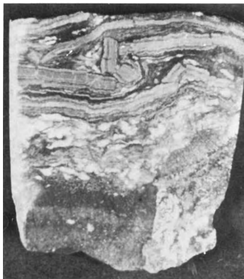
Fig. 19. Contorted and broken banded jasperoid. E bed, Tar Creek mine. One-half natural size.
