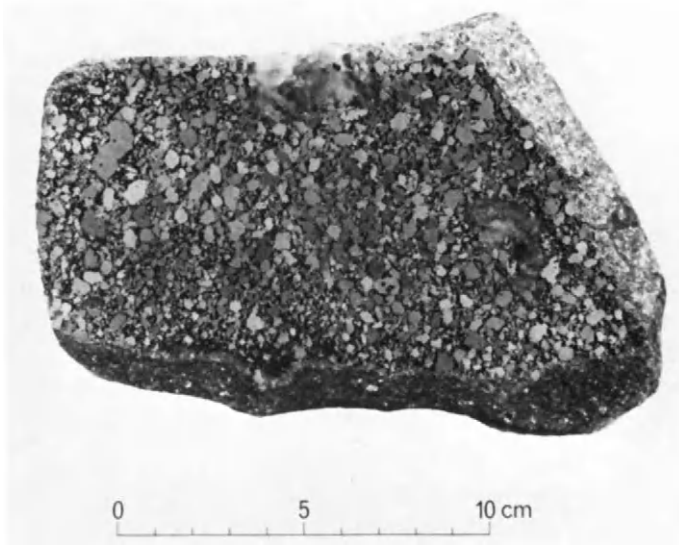
Fig. 32. Pyrite porphyroblasts in a matrix of sphalerite and pyrrhotite, Geco mine.
