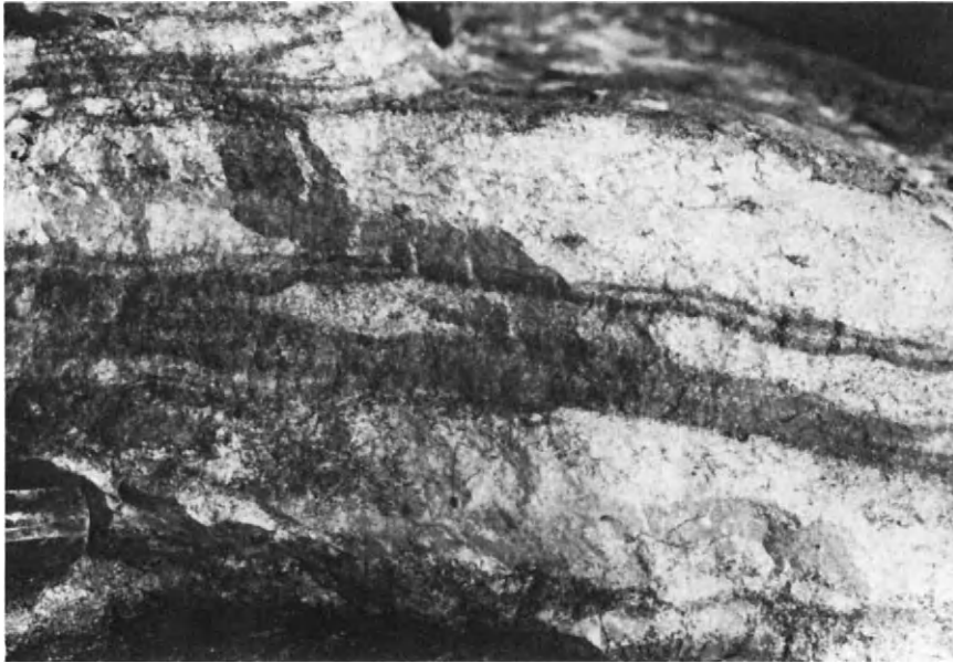
Fig. 27. Banded sphalerite (dark)–pyrite (light) ore, Mattabi mine. Head of hammer gives scale.
