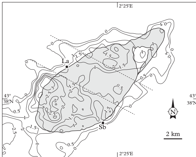
Figure 6.15 Calculated floor depth (in km) of the Sidobre pluton, showing a weakly rooted, flat-floored pluton characteristic of a sill. The poor adjustment of the calculated zero contour (with respect to the real one) is attributed to the simplistic model used for the regional anomaly as well as to local density variations due to the presence of several granite dykes in the country rocks, and to the presence of late, NW-SE directed faults (dotted). After Améglio et al. (1994). See also the map of the magmatic structures (Fig. 10.19).
