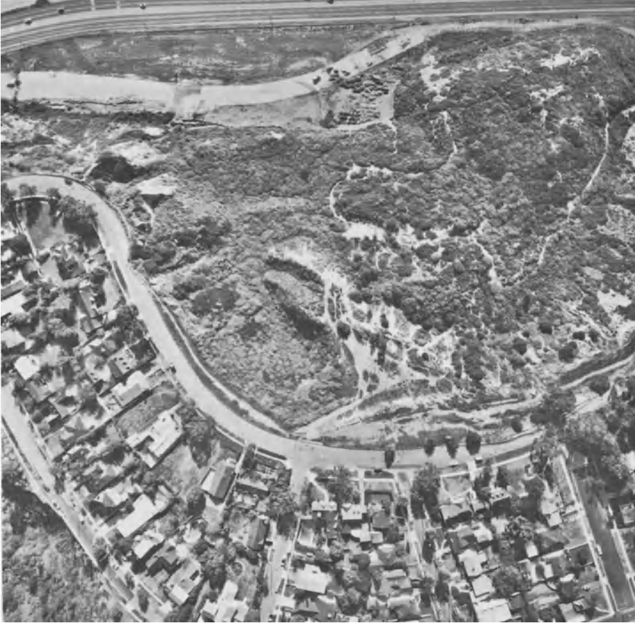
Plate 4.10. Ancient, periodically reactivated landslide, coastal highway 101, Santa Monica, Calif. The slide occupies the semi-circular area above the curving perimeter road. The relocated highway runs along the top of the photograph. (Courtesy of Pafford and Associates, Los Angeles, Calif.)
