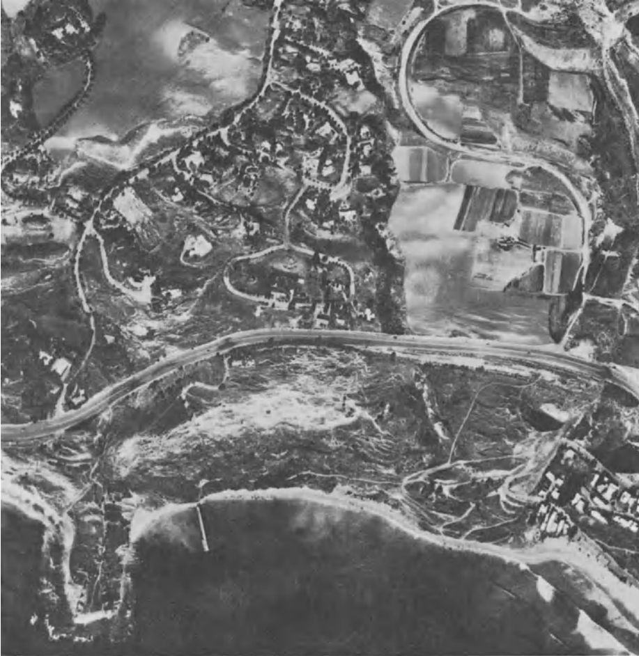
Plate 4.11. Portuguese Bend landslide, Los Angeles, Calif. The right edge of the slide lies to the left of the houses in the bottom right corner. On the left the slide is split by the rocky promontory. The rumpled topography including houses, occupying the middle of the picture is the surface of the slide mass. (Courtesy of Metrex Aerial Surveys, Los Angeles, Calif.)
