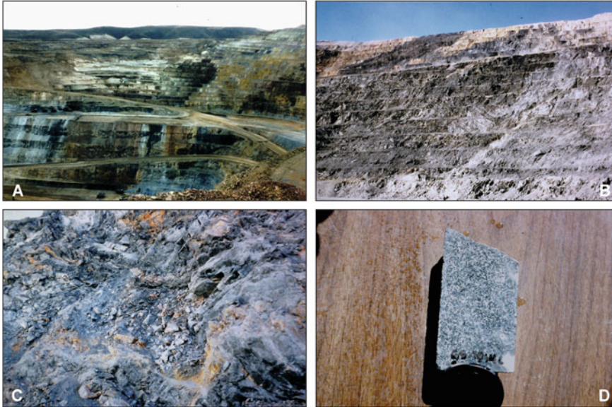
Fig. 18.5 Various rock units from in and around deposits of the Carlin Gold Province: (a) Gold Quarry open pit with bleached rocks of clays and Fe oxides overlying dark material containing arsenian pyrite and carbonaceous material. There is a wedge of Cenozoic sediment in the top centre; (b) pit highwall with upper oxidised bleached
