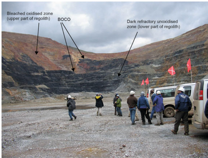
Fig. 21.6 Upper part of the regolith profile in the Gold Quarry open pit of the Carlin Gold Province. Above the base of complete oxidation (BOCO) ferric minerals convey yellow, red and orange colours; and sulfides minerals have been oxidised liberating Au and making it amenable for heap leaching. Below BOCO the dark colour reflects
