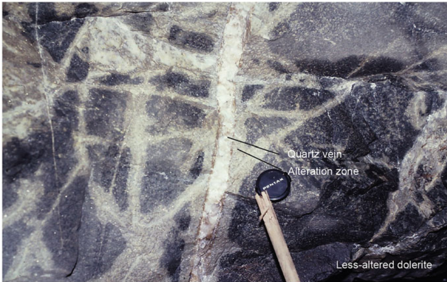
Fig. 2.3 White quartz vein (2 cm thick and vertical, left of lens cap) in dark green dolerite from Mt Charlotte mine in the Kalgoorlie goldfield of Western Australia. Numerous cream veins at various orientations are a network of
