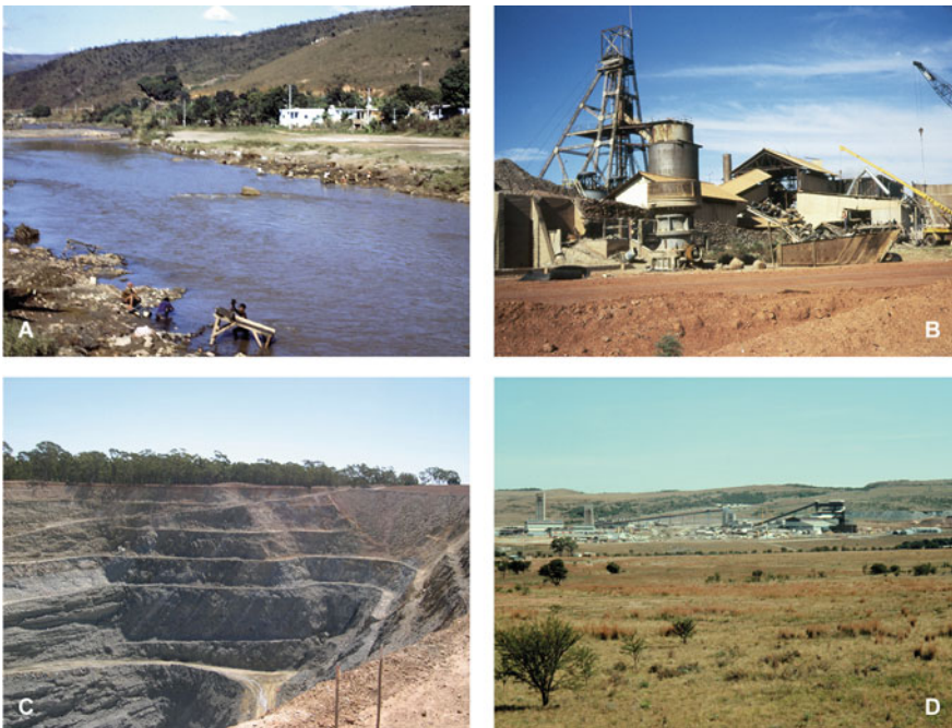
Fig. 2.2 Various styles of mining operation in the late 20 th century: (a) Several groups mining alluvial gold from a river near Cuiabá in Brazil; (b) Perseverance mine headframe and Great Boulder mill, Golden Mile, Kalgoorlie in 1982 prior to the Superpit; (c) open pit mine at Fosterville in Central Victoria [photo by Gary
