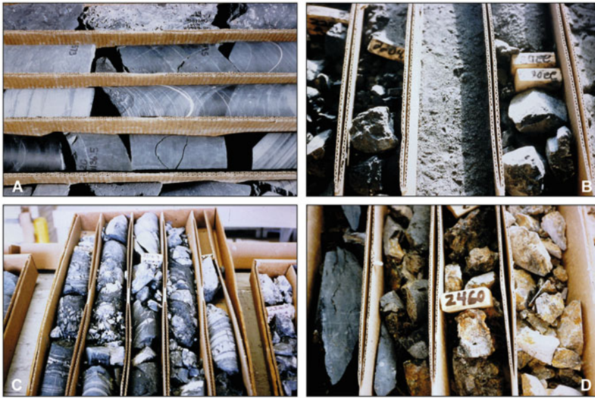
Fig. 18.4 Drill core from deposits of the Carlin Gold Province: (a) relatively intact core of metasedimentary rocks from 500 m depth as expected in most drilling deeper than ~100 m; (b-d) core from near Rain mine
