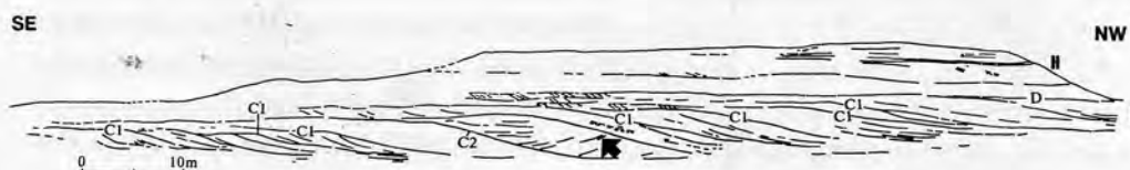
Fig.14 Detailed view of a prograding ebb-delta complex, showing the offlap pattern of two ebb-delta lobes. Each lobe consists of a depo-lobe with large cross beddings (A) and a feeding channel with an offlap stacking of megaripple sets (B). Several offlap bounding surfaces (C1) show erosion and reactivation due to stage changes or megaripple overtaking. Some reactivation surface (C2) was produced by subordinate flood currents. The ebb-delta lobe is capped by an abandonment surface (D). Arrow indicates megaripple cross-bedded set of flood currents.
