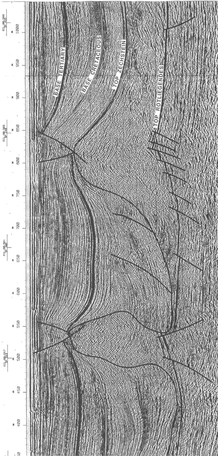
Fig. 5. Example seismic section illustrating salt effects in the basin.
