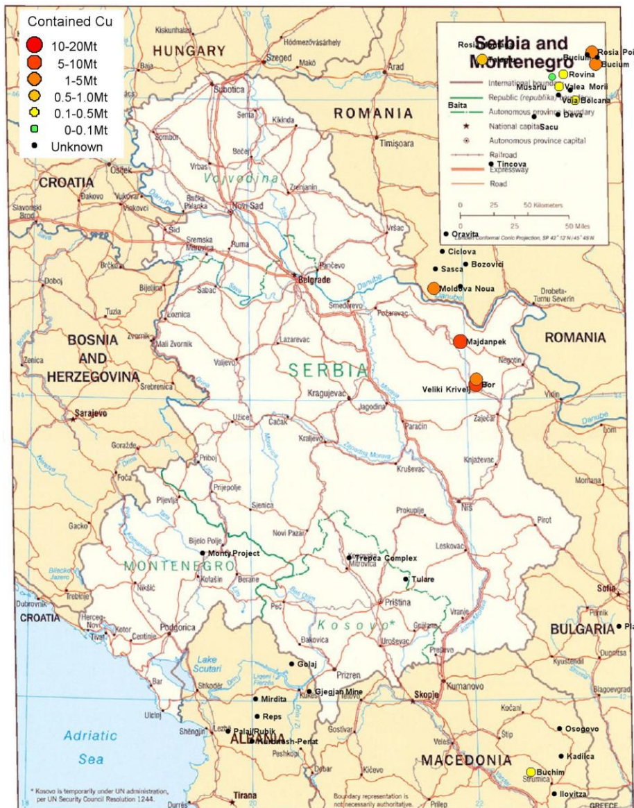
Figure 12-1 Political map of Serbia and Montenegro showing copper deposits by contained copper resources. Adapted from the University of Texas Libraries, The University of Texas at Austin (2005)
