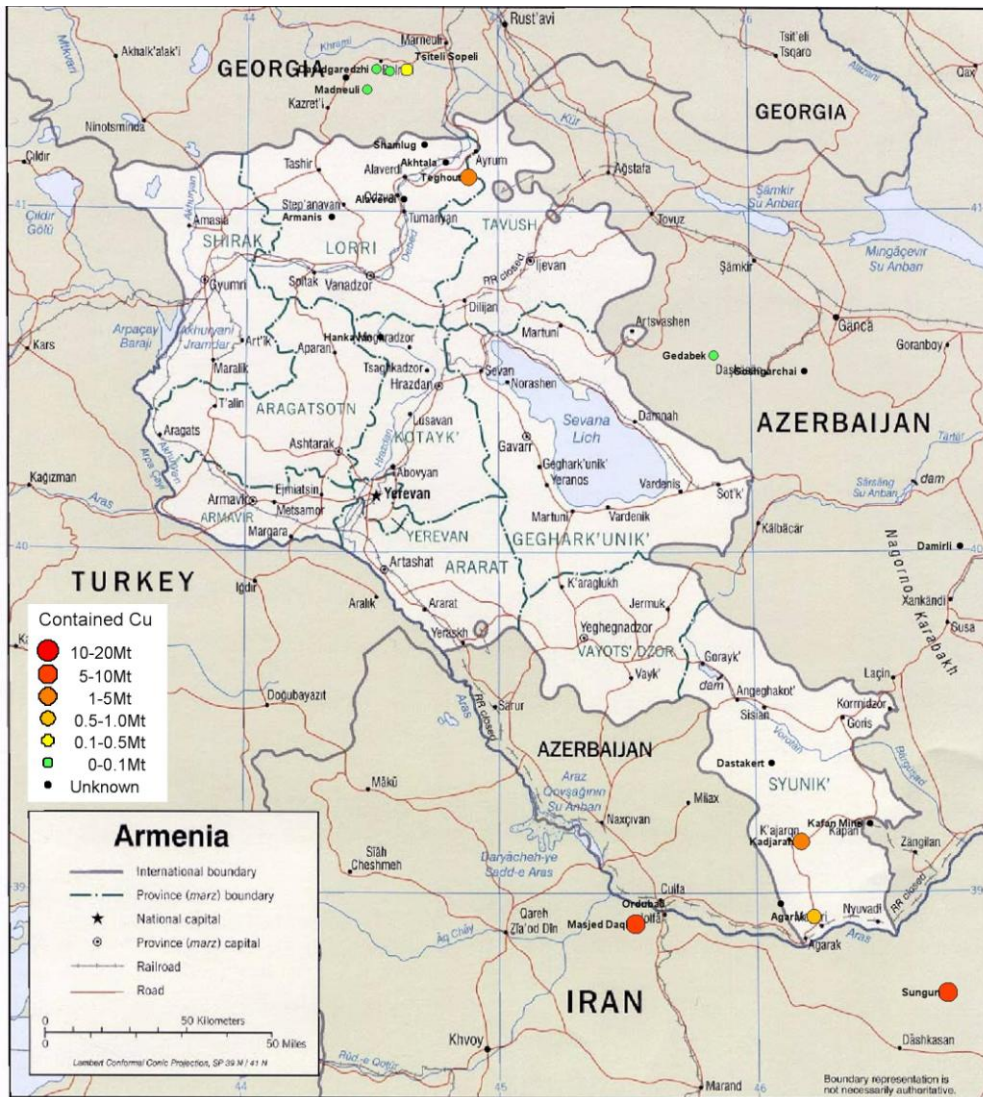
Figure 20-1 Political map of Armenia showing copper deposits by copper resources. Adapted from of the University of Texas Libraries, The University of Texas at Austin (2002)
