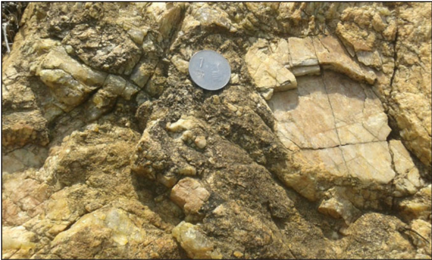
Fig. 10 Field photograph of pegmatite showing large crystals of orthoclase and quartz. The diameter of the coin is 2.5 cm. Loc. North of Sonrai
