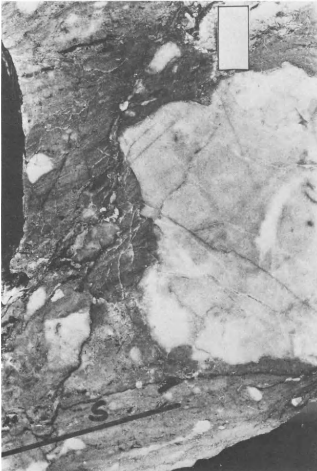
Fig. 27. Internal sediment rich in minerals in the solution cavity of the cataclastic Wetterstein Dolomite. The internal sediment contains as fine bedding (s) varying amounts of sphalerite, galena, pyrite, marcasite, quartz, fluorite, baryte and dolosparite, as well as resedimentated dolomite rock detritus from the cavity ceiling. “Westschachtscholle”, Bleiberg-Kreuth mining complex. Plain section, 1-cm scale with mm-divisions.
