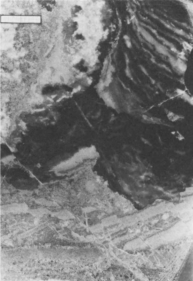
Fig. 21. The mechanical inhomogeneity becomes obvious through syndiagenetic deformation of the sphalerite sediment. Bituminous-clayey calcilutite is crumpled (center of picture and upper right), recrystallized rigid ZnS-crysts in the sphalerolutite are broken. Wetterstein Limestone, Lafatsch Mine. Plain section, 1-cm scale with mm-divisions.
