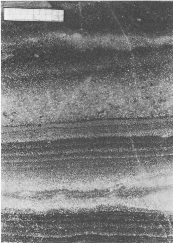
Fig. 4. Polar fabric formed by space-rhythmic apposition of sphalerite (fine-grained, light grey) in calcilutite. Repeated sequences of strong increase and decrease in ore content with height. Wetterstein Limestone, Lafatsch Mine, Tyrol. Plain section, 1-cm scale with mm-divisions.
