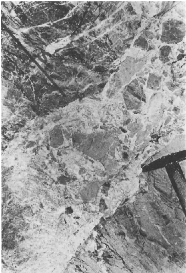
Fig. 24. Vein unconformable with respect to stratification in Middle-Triassic Wetterstein Limestone, brecciated, with dominating baryte-mineralization (white). Deformation and mineralization turned out to be syndiagenetic. Rudolf Mine, Bleiberg mining complex.
