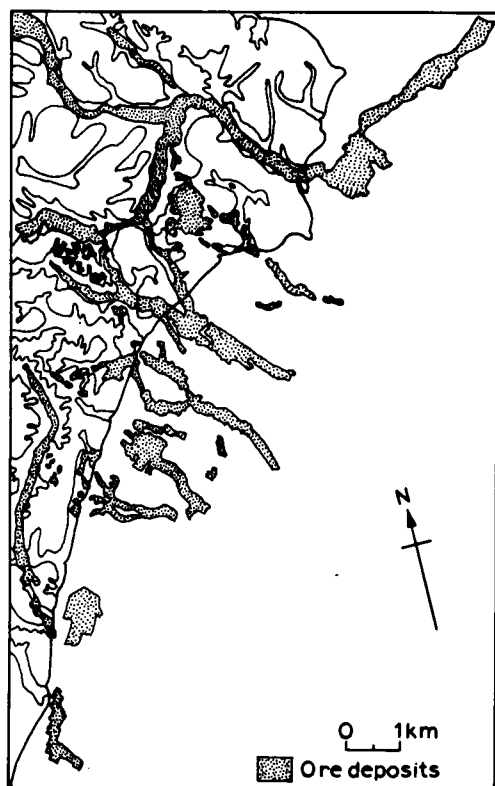
Fig. 6. Tin ore deposits in old river valleys on land and nearshore. East coast of Singkep, Indonesia. (From Zaalberg, 1970.)
