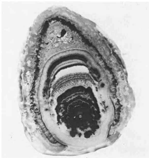
Fig. 5. Polished surface of a cross-section from a composite stalactite, about 2.5 \times natural size (Djebel Hallouf, Tunisia). Whitish = calcite–aragonite; dark grey to black = galena; white = empty spaces.
