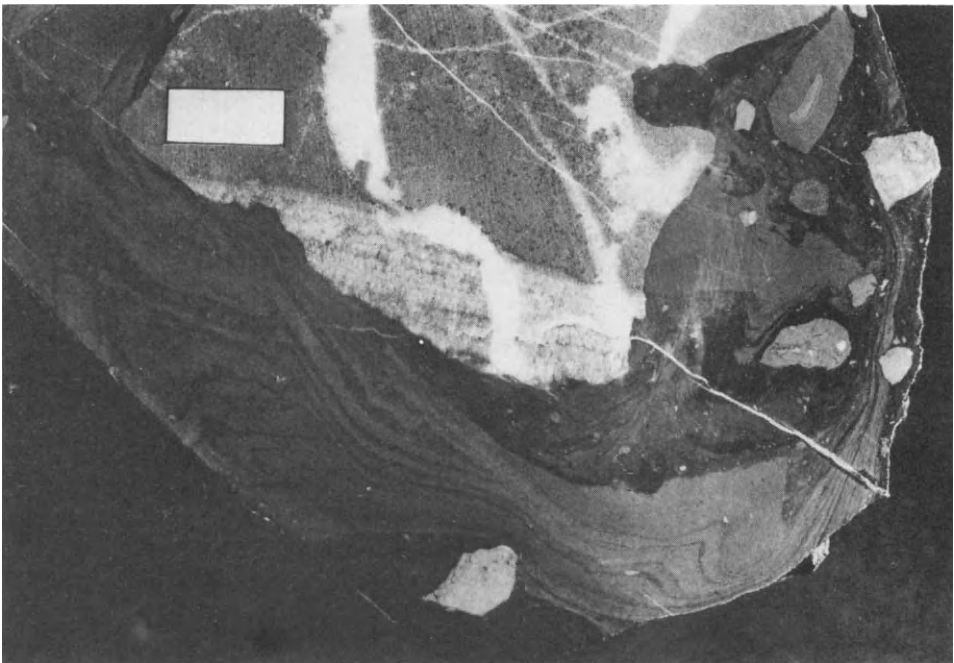
Fig. 13. Subaquatically deformed, finely bedded rhodochrosite-lutite in a sedimentary-brecciated part of the manganese deposit Dawin-Alpe, Lechtal Alps, Tyrol. Plain section, 1-cm scale with mm-divisions.
