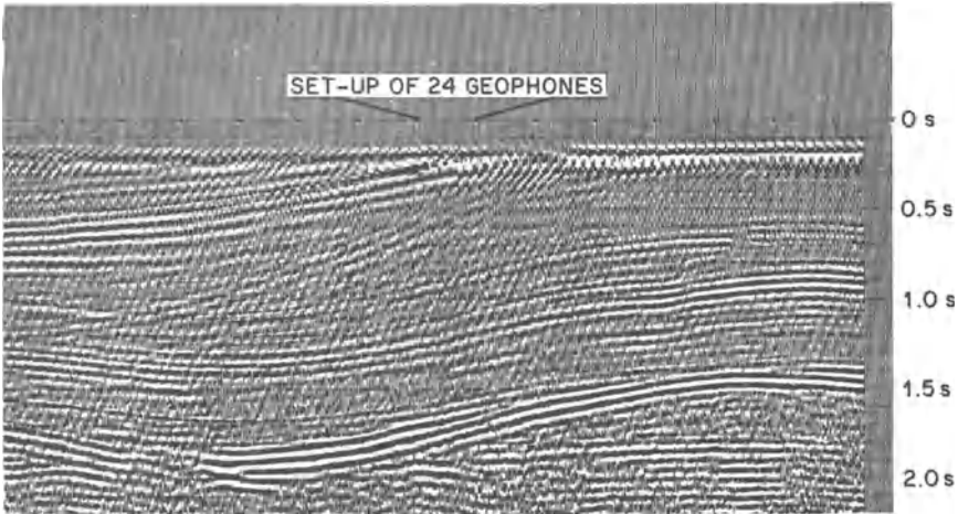
Fig. 7.27 Display of juxtaposed VAR records from consecutive geophone set-ups. Each geophone trace is a CDP stack of signals as explained in the text. (Courtesy of Seismograph Service Ltd. Holwood, England, and Amoco/Gas Council North Sea group.)
