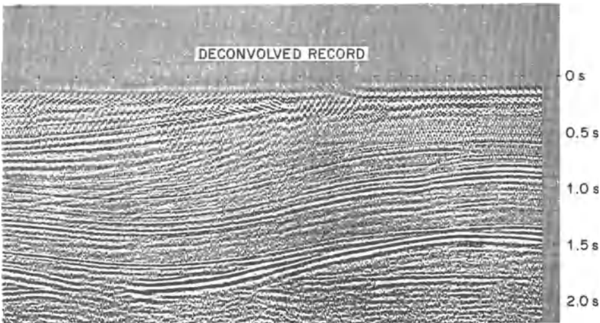
Fig. 7.28 Section of Fig. 7.27 after deconvolution. (Courtesy of Seismograph Service Ltd. Holwood, England, and Amoco/Gas Council North Sea Group.)
