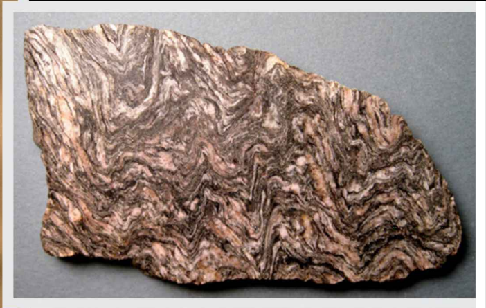
A sample of migmatite, a metamorphic rock with light and dark bands of minerals and folding due to exposure to high temperatures and intense pressure deep within the earth's crust (see Chapter 7).
