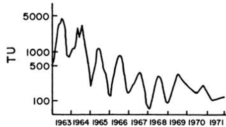
Fig. 10.5 Summer peaks and winter lows of tritium observed in precipitation in Sweden. (From Pearson, 1974.)
