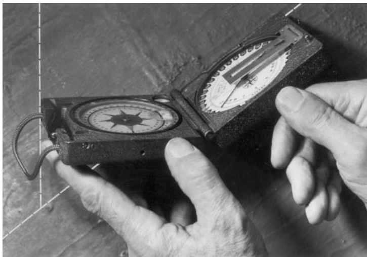
Figure 5.13 Measuring lineation on a steep surface using a compass with a hinged lid
