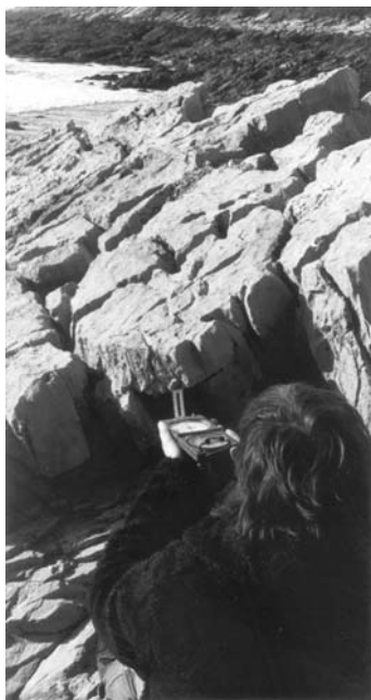
Figure 5.5 Measuring the strike of an uneven surface with a prismatic compass (Method 3)
