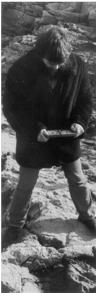
Figure 5.3 Measuring the strike of a veinlet on a rough horizontal surface by Method 2
