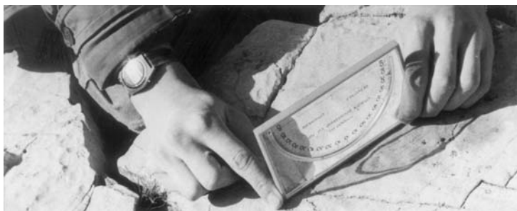
Figure 5.2 Using a 'Dollar' type clinometer to measure dip
