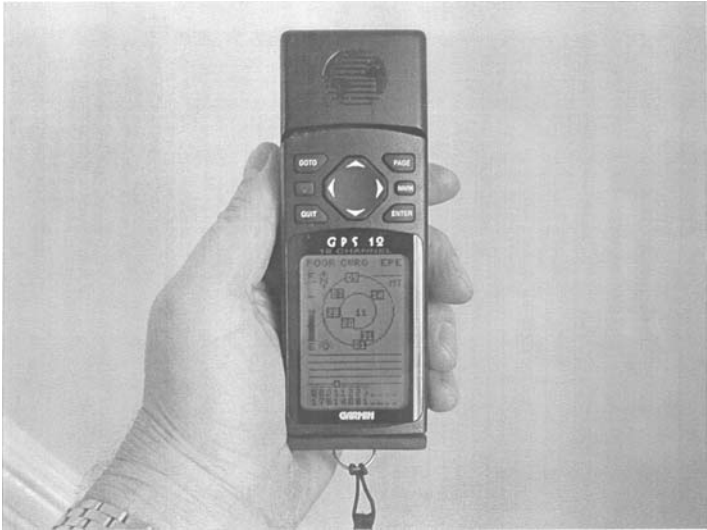
Figure 2.11 A Garmin GPS-12, typical hand-held GPS instrument. It can locate you to within a few metres on the ground and assist you in following a specific route. It cannot be used in forest because it requires a clear view of several satellites. It also does not function well in icy conditions
