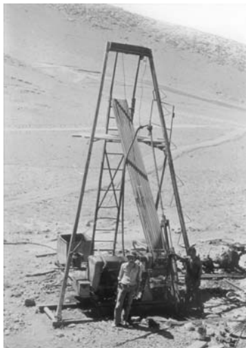
Figure 4.8 A diamond drill rig drilling an inclined hole
