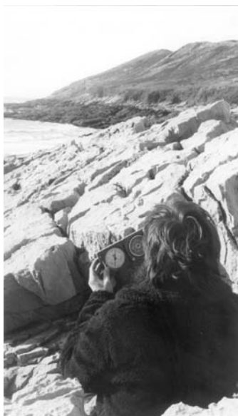
Figure 5.6 Measuring the dip of an uneven surface by Method 3
