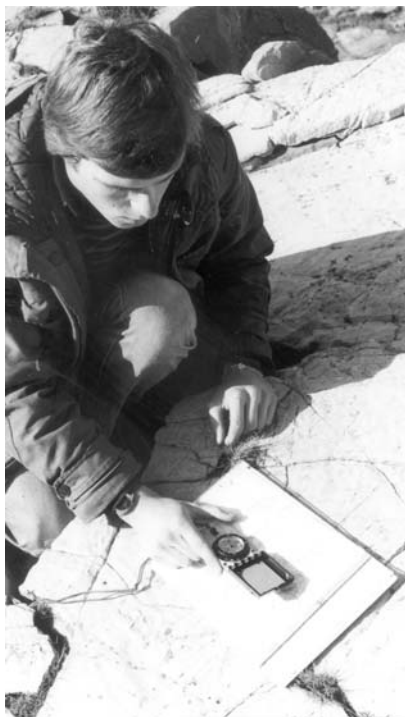
Figure 5.1 Measuring strike by the contact method
