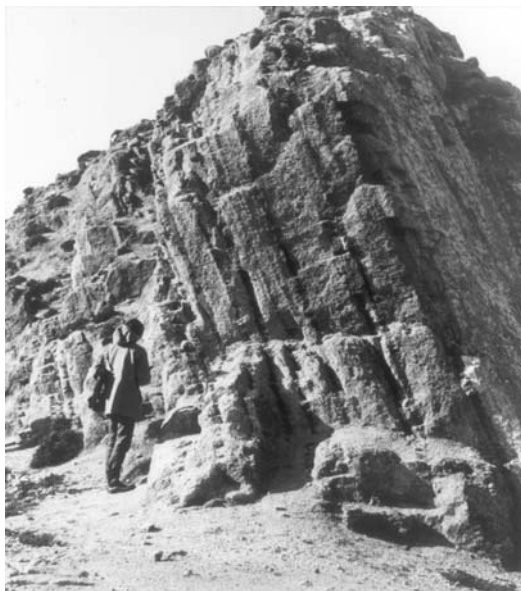
Figure 5.4 An ideal exposure for the end-on measurement of dip
