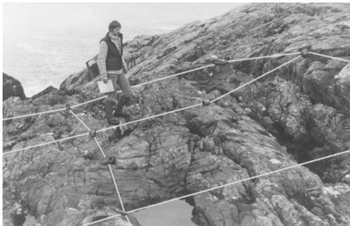
Figure 4.12 A 4 m mesh cord grid to aid sketch mapping laid over an exposure at Badcall, NW Scotland (see Figure 4.13); the cord has been retouched for clarity
