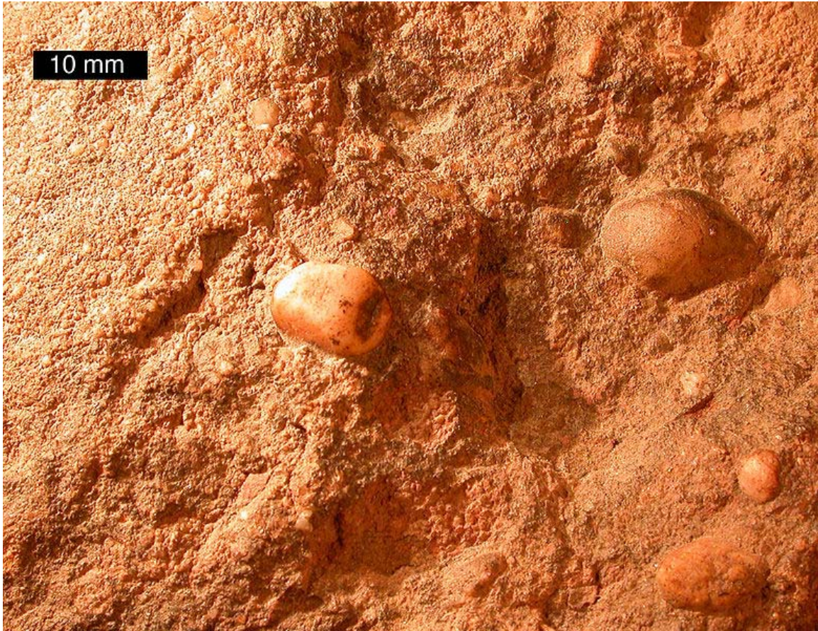
Bedding plane of Old Red Sandstone with quartz and chert pebbles; central England; (scale bar is 10 mm.)
