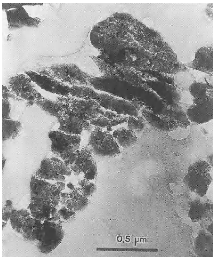
Fig. 9. Transmission electron micrograph of an ultrathin section of chondritic IDP L2011K7 embedded in epoxy (gray background) showing fusion of subspherical (carbon-free) ferro-magnesian-aluminosilica (very low \text{Al}_2\text{O}_3 ) units with ultrafine-grained Mg, Fe-olivines and pyroxenes and iron oxides. The shattered appearance is an artifact of ultramicrotome sectioning
